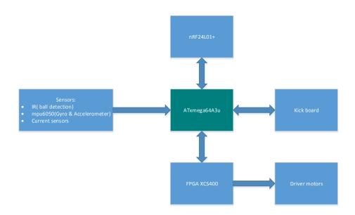
Fig. 2. Block diagram of the electrical system.
