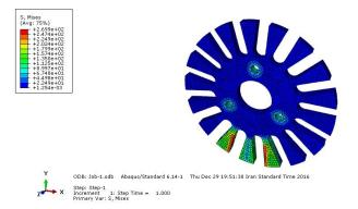
Fig. 4. The wheel's hubcap after considering the forces between hubcap, pitch, and screws.
