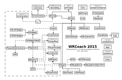
Fig. 4. Simplified diagram of the modules of the WRCoach software.
