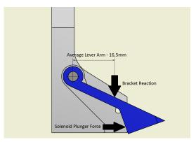
Fig. 7. New Chip Kick Diagram
