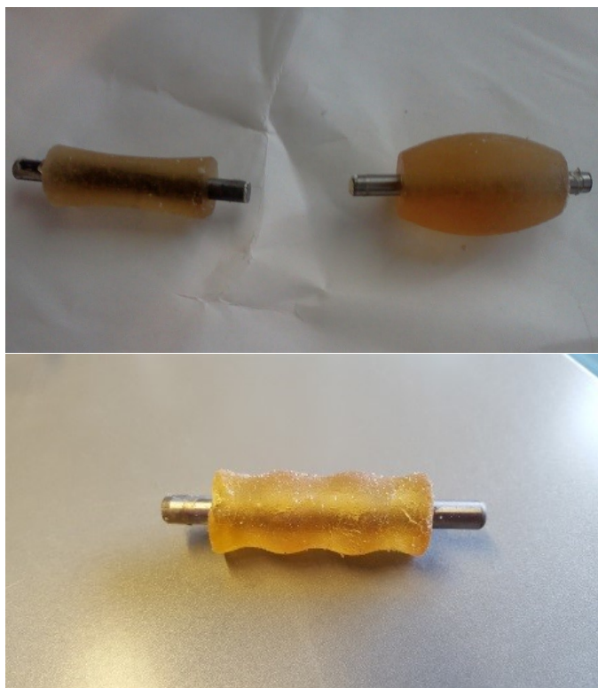
FIG. 2. The convex, concave, and sine wave finished casted parts. Notice the rough edges on the dribblers.
