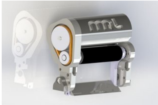
Fig. 19. New dribbling system of the MRL robot
