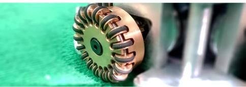
Fig. 2. Omni-directional wheel structure.
