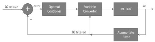
Fig. 4. Torque controller [6] block diagram
