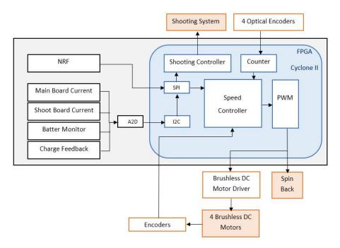
Fig. 3. Robots Hardware Block Diagram.
