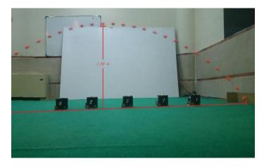
Fig. 6. Chip kick test in laboratory
