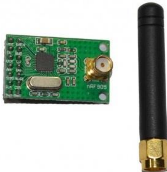
Figure 2: Image of NRF905 Wireless Module [1] .
