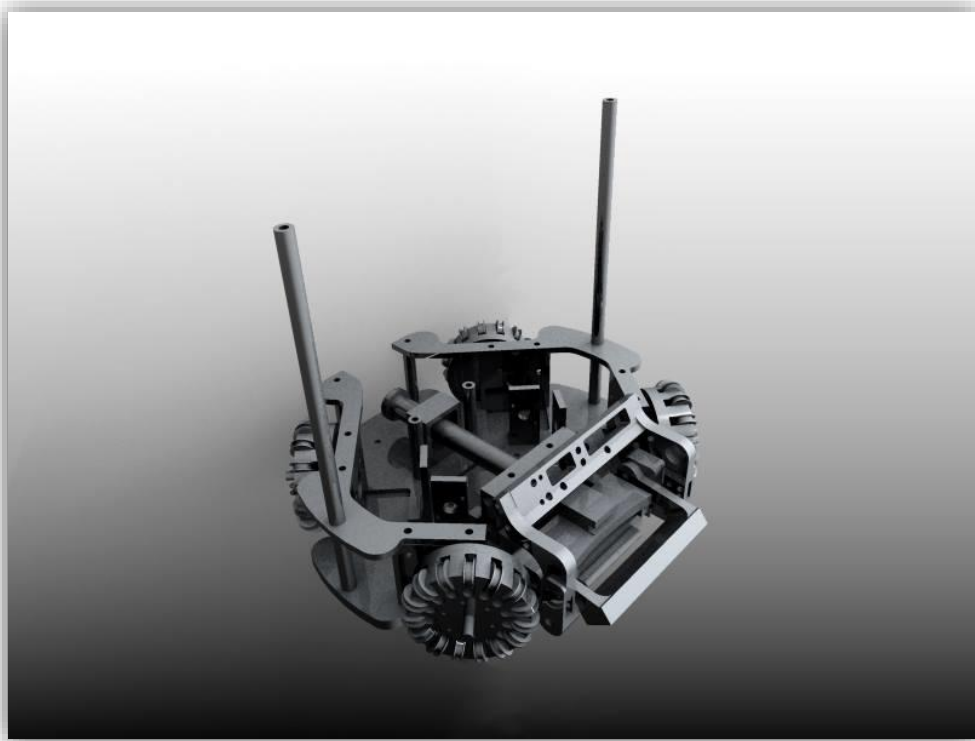
Figure 4: 3D Design of Complete wheel assembly and Chasses.
