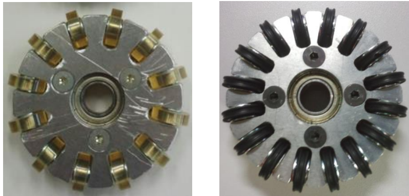
Fig. 1 Wheel of 2014 model (left) and 2015 model (right)
