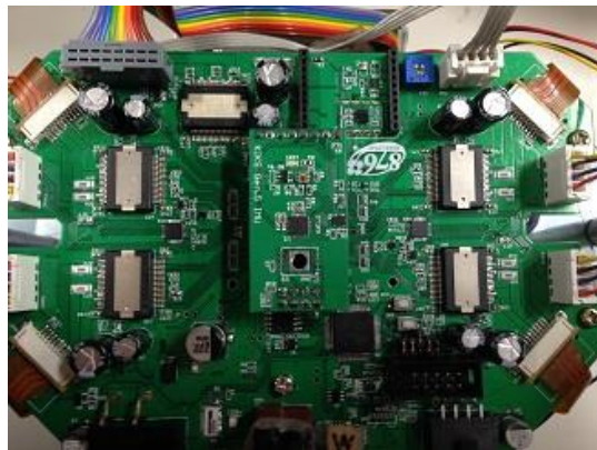
Fig. 6 IMU circuit mounted on FPGA
