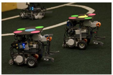
Fig. 5. Lego NXT Robots used for initial development
