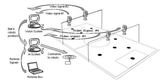
**Fig. 1.** Typical architecture of a SSL team.
