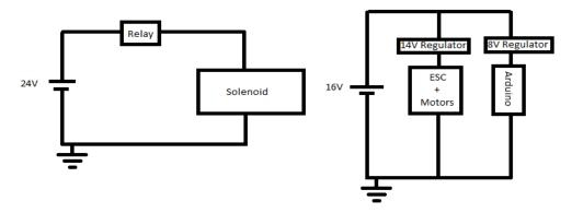
Fig. 4. Power supply to robot components
