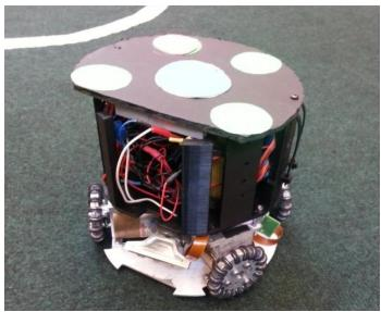
Fig. 3. First generation RoboBulls SSL robot.
