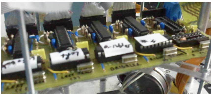
Fig. 5. Motor control board
