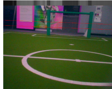
Fig. 1. Image showing the horizon band. The single row of grey-scale pixels taken from the horizon band for landmark extraction is shown at top of image.
